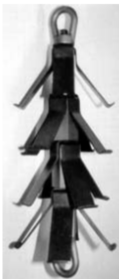
Figure 1.2. Pipeline cleaning equipment with brush or chain drives
